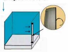
Position the vertical closing profile 2 as indicated in the image of the circle, with the L-shaped part facing out.
