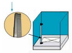
Remove the protection of the vertical closing profile and fix it on the wall.
